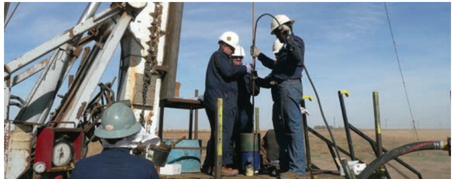
SCS proof-of-concept trials sucker rod deployment
