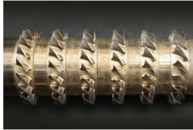
SCS Compressor Blades after the Trial (Rust Shown in Picture was Pipe Debris Moving through the Compressor)
